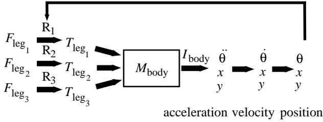
Figure 17. Feedback through the mechanical system. Leg ground-reaction forces ( $F$ ) act by way of moment arms ( $R$ ) to generate a torque ( $T$ ). Torque on a body of a given mass ( $M$ ) and inertia ( $I$ ) produce a rotation ( $\theta$ ), sideways ( $x$ ) and forward ( $y$ ) translation. Feedback in this feed-forward system results from the effect of position on the moment arms.
