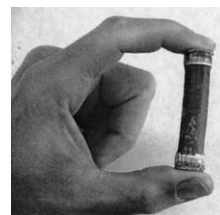
Figure 1. A spring roll with axial extension strain. It was fabricated by rolling two prestrained about a compressed central spring.
