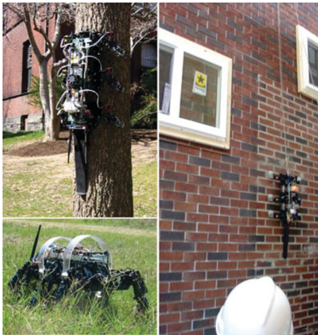
Figure 7. The RiSE platform is capable of scaling a wide variety of real-world surface types and variations as well as maintaining capable level-ground locomotion. Clockwise from the upper left, RiSE climbing a tree, climbing a brick wall, and walking through tall grass.
